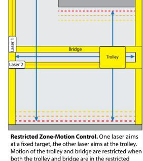
at a fixed target, the other laser aims at the trolley. Motion of the trolley and bridge are restricted when both the trolley and bridge are in the restricted zone, effectively preventing the crane from entering that area. Three sets of alarms control Bridge Forward, Bridge Reverse, and Trolley Forward. The relay outputs are wired in parallel to ensure movement is restricted only when the bridge AND trolley are in the restricted zone.
