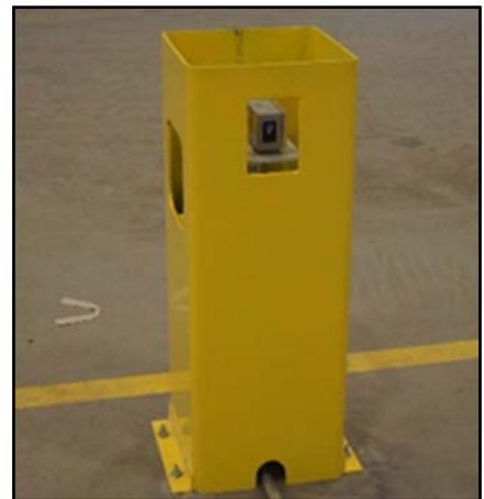
Dimetix laser and protective housing.
