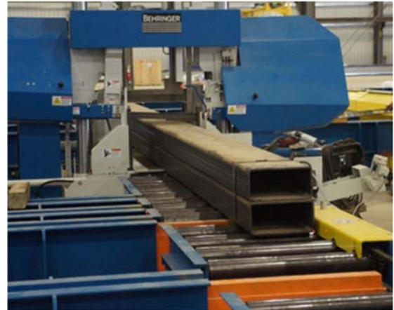
Behringer saw controlled by DIMETIX USA cut-off system.
