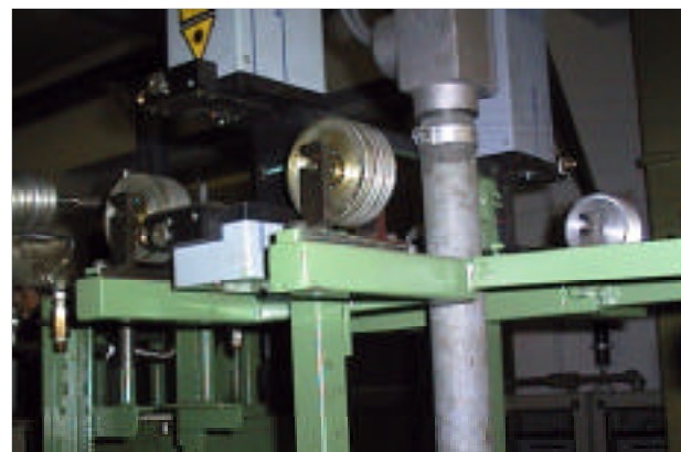
Pictured above is an installation of a Wirescan system. Two Wirescan 40 systems are depicted. One in the foreground and one in the background. To the right is a block diagram of a typical Wirescan system. It illustrates three remote displays, three electronic potentiometers, and a PC connected to the RS 485 port. Two printers can be supported since one printer is connected directly to the IBU control unit. Compressed air windows can be bolted to the ALS 40 laser gauge head for operation in dirty environments.
